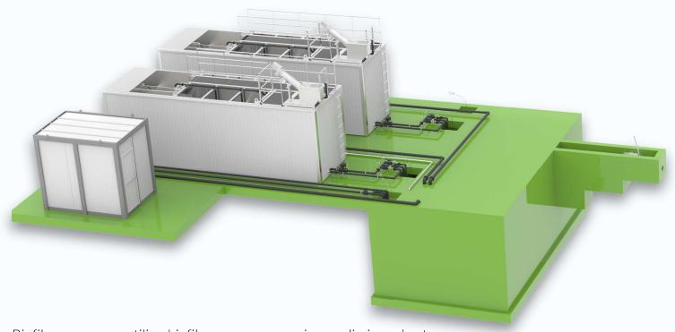
Biofilm processes utilize biofilm grown on carrier media in order to aerobically degrade soluble organic pollutants in the wastewater. These applications typically include a biological reactor filled with floating biomass carriers, a screen to prevent downstream migration of the carriers and an aeration grid. Different configurations may apply to address various scenarios.
